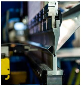
Maximum bending pressure: 313 kN Maximum force to support the sheet: 509 kN Maximum height of bending: 350 mm Maximum bending inside: 55 mm Minimum dimensions for pieces for bending: 200x400 mm2 Maximum dimensions for sheet formats: 1,500x2,160 mm2 Max. opening (max. distance between pressed&bending blade): 350 mm Max./Min. thickness of material: 2/0.8 mm
